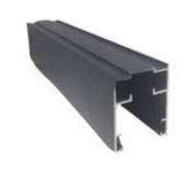
Heavy duty aluminum while most rolling screen are made of aluminum profile of 0.6-0.8mm,our system insist to offer 1.2mm-1.5mm for different section to make a strong body.
